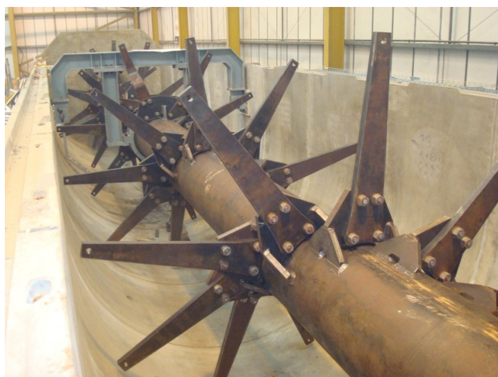
HotRot 3518 central tine bearing shaft – unit lids removed
