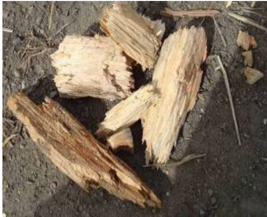
Oversized shredded timber >50mm in size.
