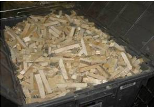
Sawn timber off-cuts 10-20mm wide x >50mm long.
