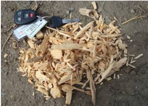
Ground waste timber – key approx. 7cm long
