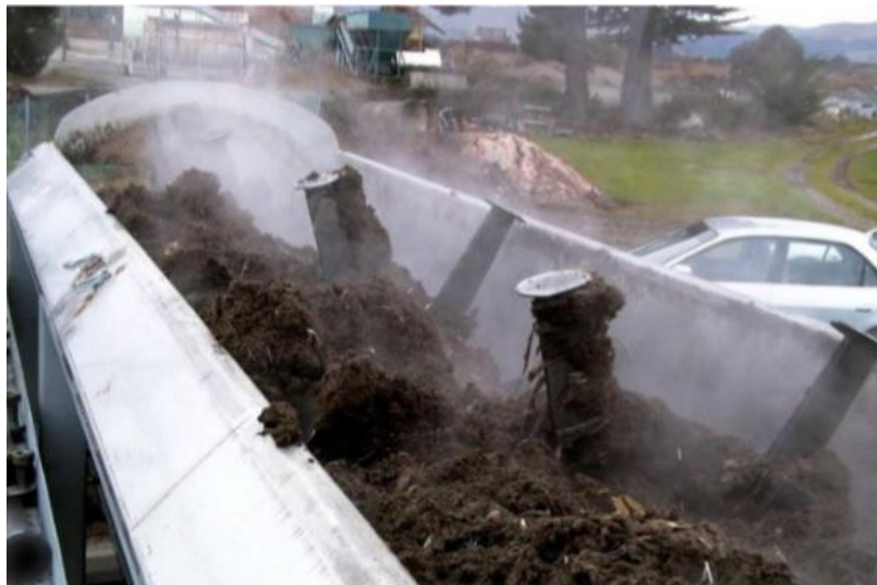
HotRot units with lids removed showing release of moisture and gases during shaft rotation.
