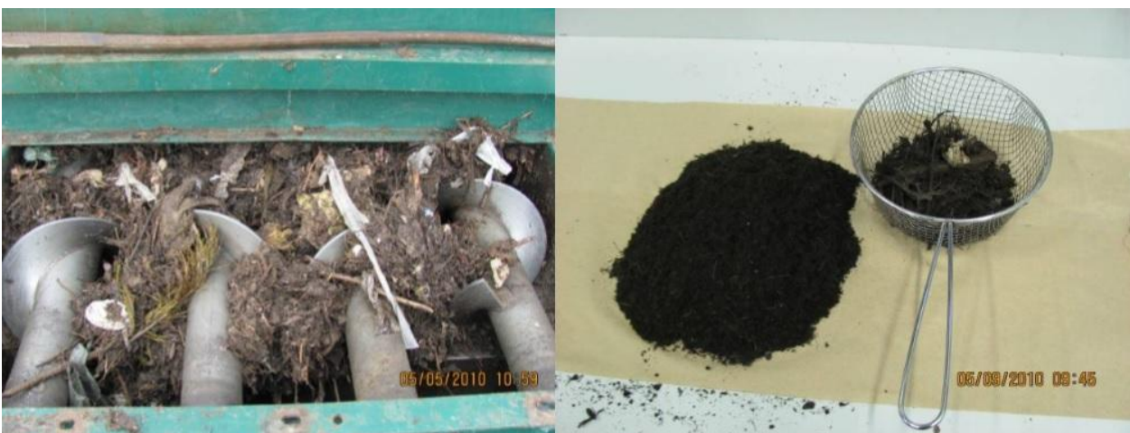
Day 0 – Waste in feed hopper(left). Day 5.5 – Product from HotRot screened.
