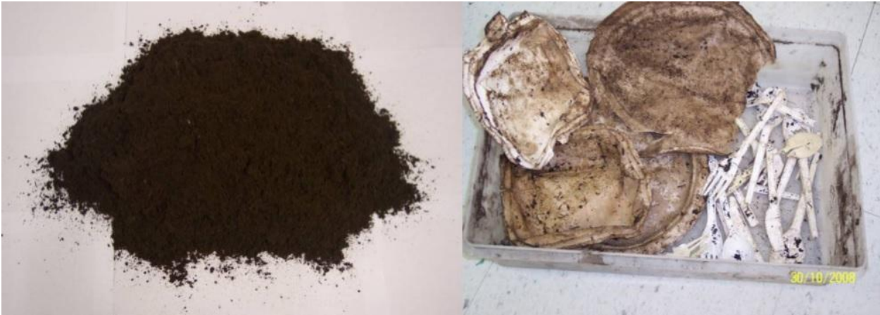
Compostable tableware after 10 days in a HotRot composting unit (left) and after 10 days in aerated container (right).
