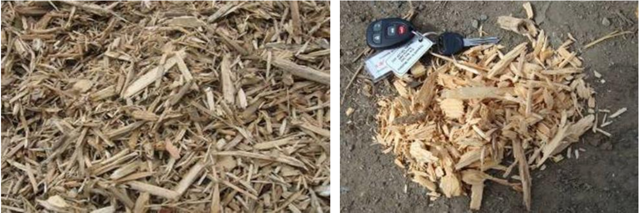
Chipped (left) and ground (right) waste timber (key approx. 70mm)
